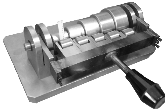
Fig. 1. The experimental device for determination of the springback angle
