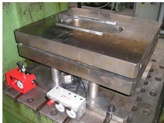
Fig. 4. The drawing die with flat restriction bars
