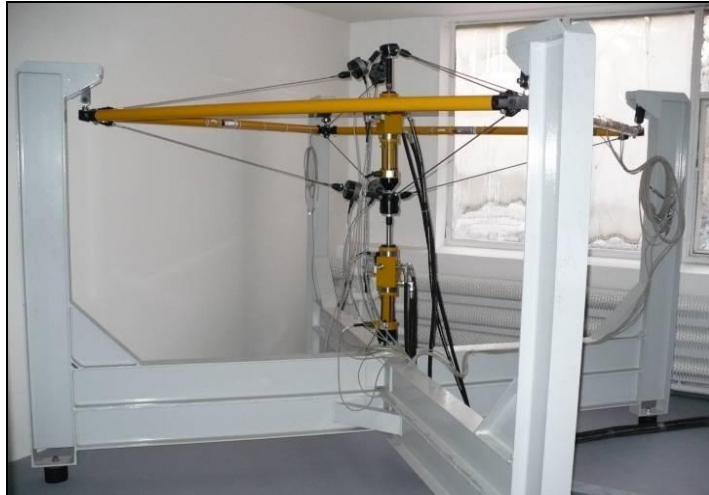
Fig. 1. The active tensegrity unit suspended on the self-supporting frame
