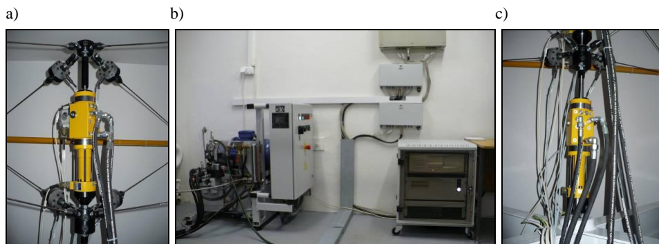
Fig. 2. Some parts of the test facility: a) action member (AP), b) hydraulic power unit, and control electronics, c) hydraulic load cylinder (ZV)
