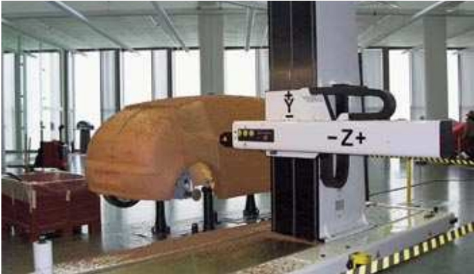
Fig. 9. A maquette production 1:1 on CNC machine in development centre PSA [8]
