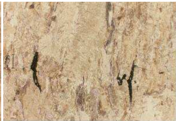
Fig. 12. Detail of cracks of sample B2
