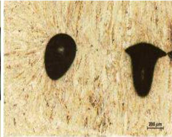
Fig. 10. Detail of cavities in the middle of weld nugget of sample B1
