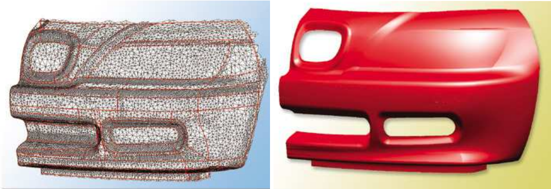
Fig. 11. „Cloud of points“ with a triangular net and smoothed surface model in ICEM Surf [7]
