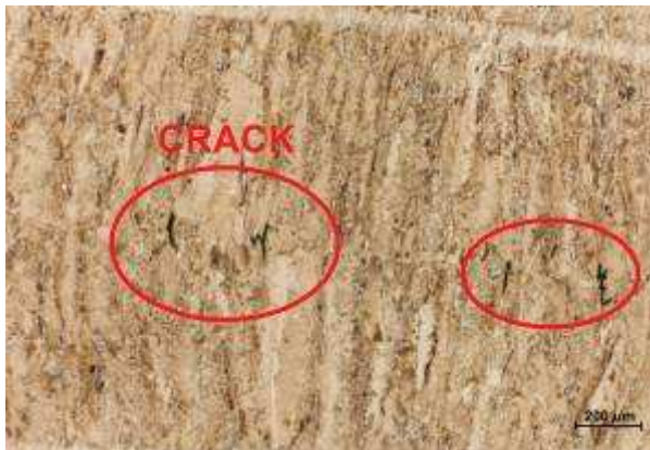
Fig. 11. Hot cracks in microstructure of sample B2
