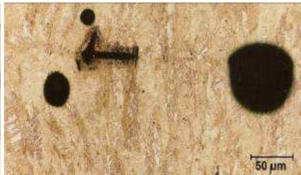
Fig. 16. Details of cavities in the middle of weld nugget of sample D1
