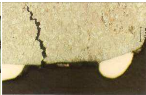
Fig. 18. Intercrystalline crack in HAZ on sample D2
