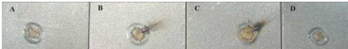
Fig. 3. Welding electrodes indentations on TRIP steels
