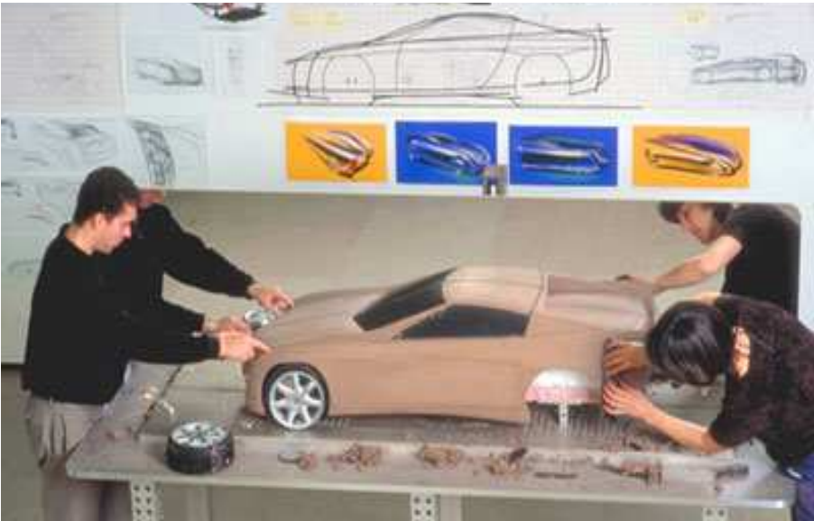
Fig. 10. Making a clay model [10]
