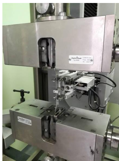
Fig. 2. An example of a sample during the uniaxial tensile test
