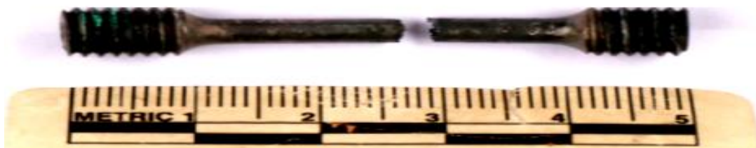
Fig. 11. Sample cut from the P9 blade - the sample after the creep resistance test broke after 52.6 h.
