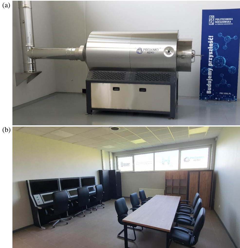
Fig. 4. Images showing the existing burner rig (a) and the control panels (b).
