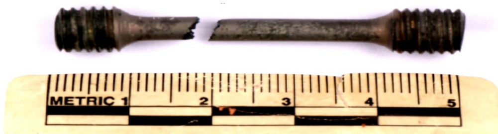
Fig. 10. Sample cut from the P4 blade - the sample after the creep resistance test broke after 42.6 h.
