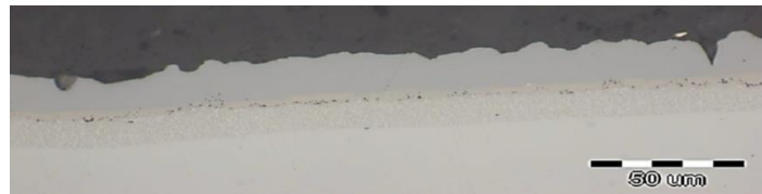
Fig. 2. Microstructure of the aluminized layer; non-etched microsection treated with Kalling's reagent (blade's suction side).
