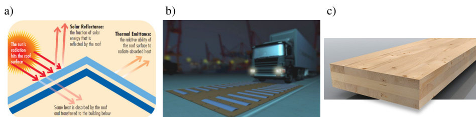
Fig. 1. Green technologies: a) Cool roof, based on [7]; b) Electro kinetic road ramp, based on [8]; c) Crosslam timber/CLT, based on [9]
