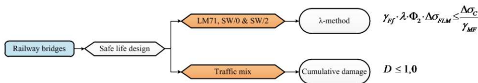
Fig. 3. Fatigue design procedure of railway bridges, acc. to [6]
