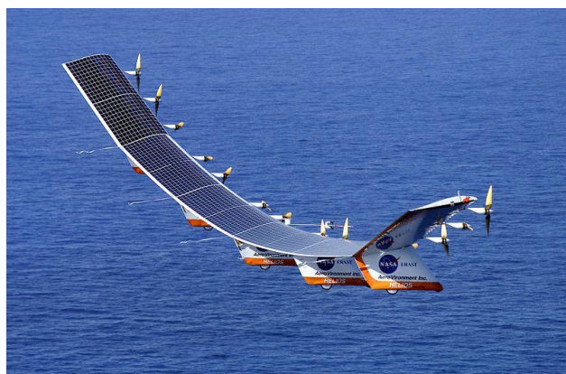
Fig. 5. Unmanned plane Helios with photo-cells on wings
