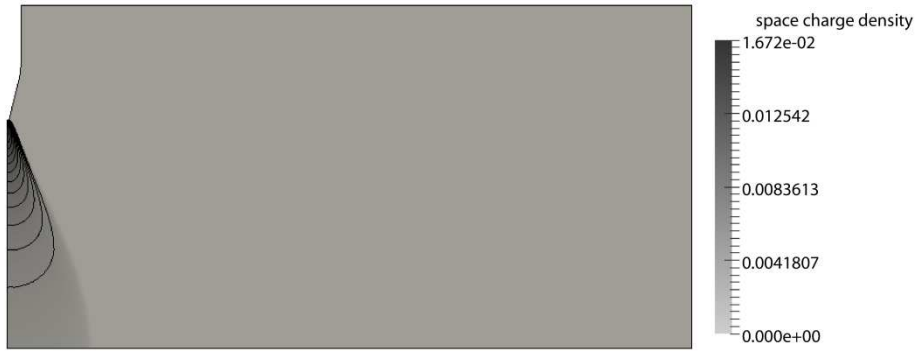
Fig. 4. Distribution of space charge density in C/m 3
