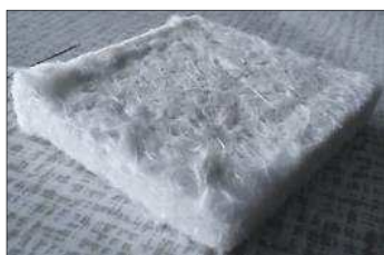
Fig. 3. The real view of the investigated sample of aerogel blanket required for Poensgen apparatus
