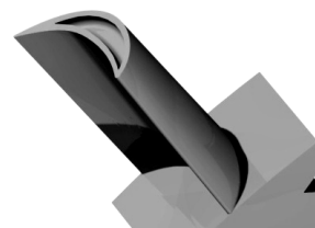
Fig. 1. Model of blade with the tip chamfering
