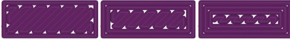
Fig. 3. Number of outline contours factor visualization for sample with orientation A with one (a), two (b) and three (c) outline contours
