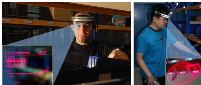
Fig. 3. Example of Pick-by-Vision, according to [5]
