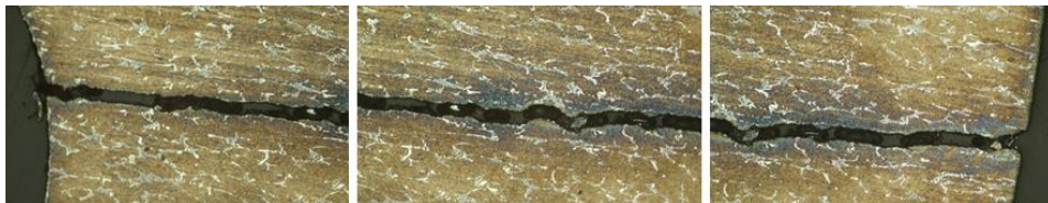
Fig. 7. Progress of cracks across the ejector wall thickness
