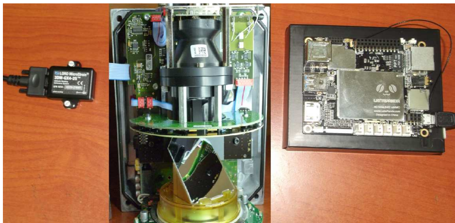
Fig. 2. A set of three basic elements tested of the remote laser scanning terrain system
