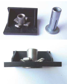
Fig. 22. Blind rivet nut with cut cylindrical flange
