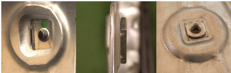
Fig. 19. The rectangular nut pressed in the vehicle window lifting element
