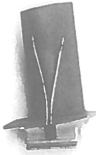
Fig. 1. A compressor turbine blade with a strain gauge sensor
