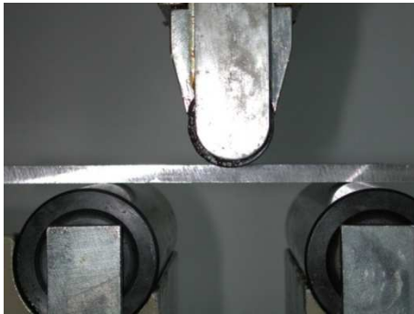
Fig. 3. Scheme of the three rolls bending test
