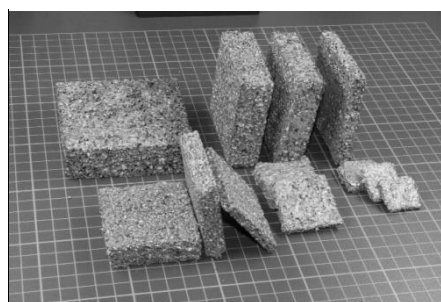
Fig. 4. Foams produced at the Maritime University of Szczecin (AlSi9/SiC composite)
