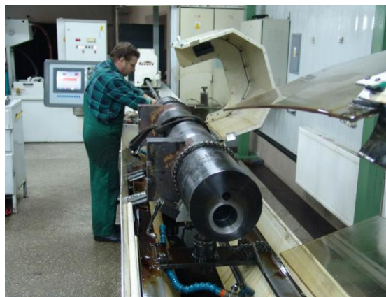
Fig. 13. Honing of large dimension cylinder
