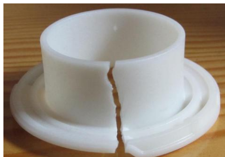
Fig. 1. The bushing damaged during assembly
