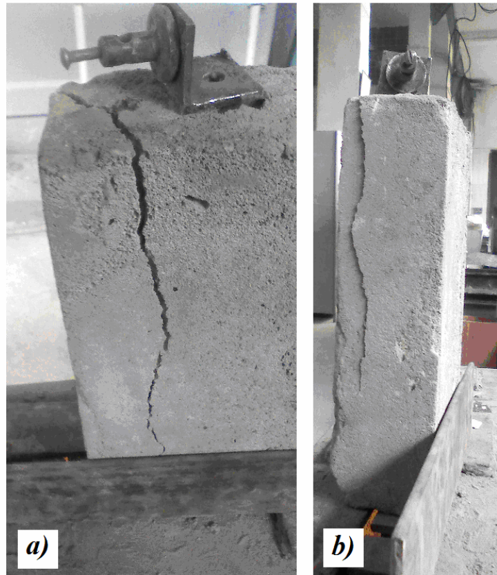
Fig. 5. The view on results of thrust effect in action: a, b) specimens splitting under the action of transversal pressure.
