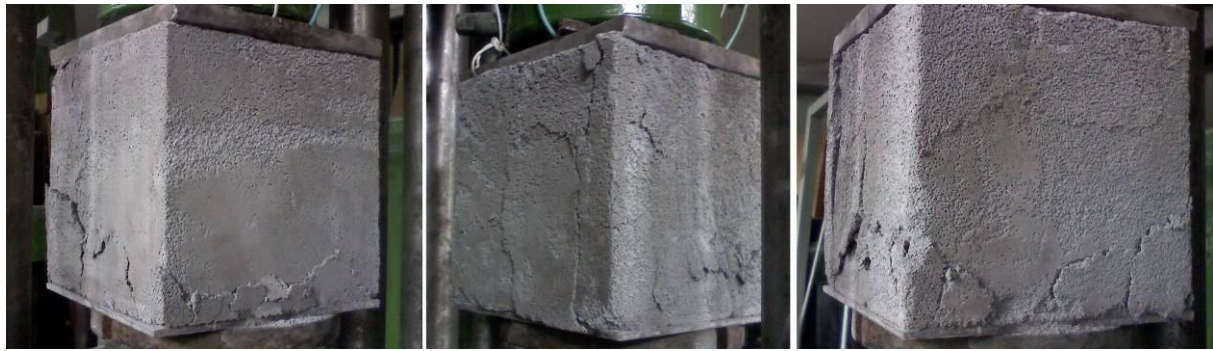
Fig. 2. The character of specimen's destruction for determination of foam concrete cube strength.
