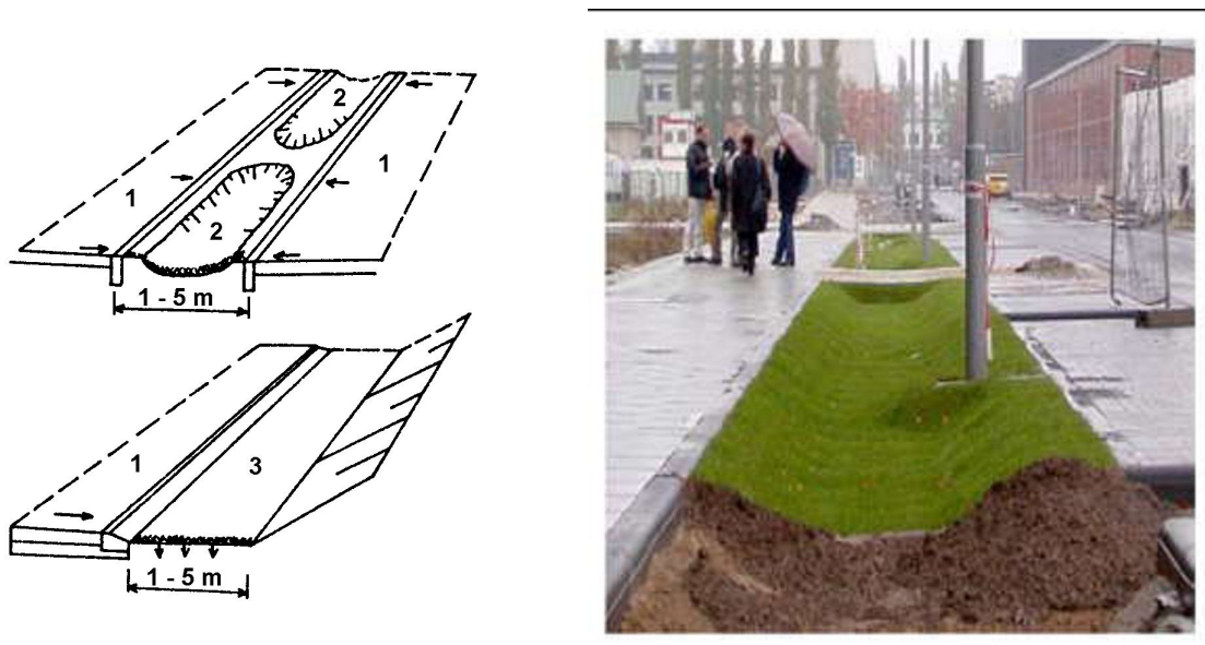
Fig. 1. Infiltration trenches 1-paved area, 2-trench, 3-green infiltration belt
