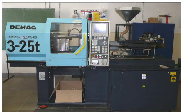
Fig. 1. Injection moulding machine - DEMAG
