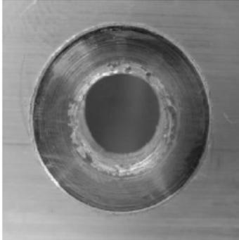
Fig. 11. Removed collar and bushing with threads
