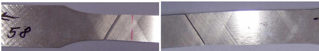
Fig. 4. Significant slip planes in two directions in respect of loading direction of tested sample
