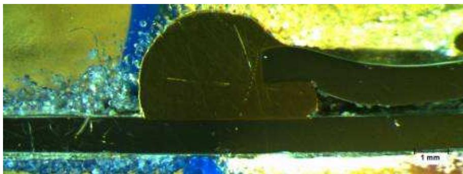
Fig. 5. Macrostructure of brazed joint of the sample F6
