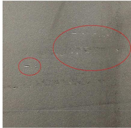
Fig. 2. Visual evaluation –impression after rolling
