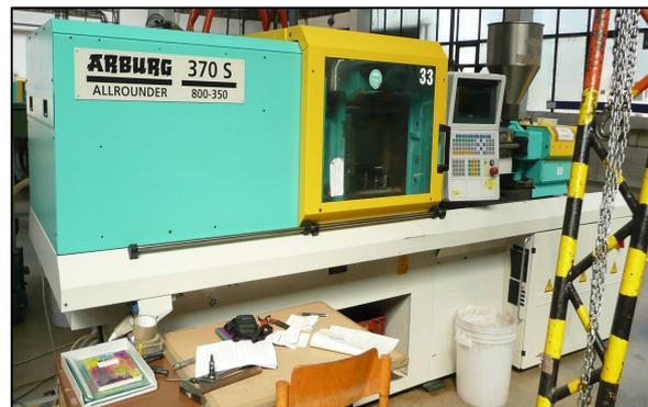
Fig. 2. Injection moulding machine - ARBURG
