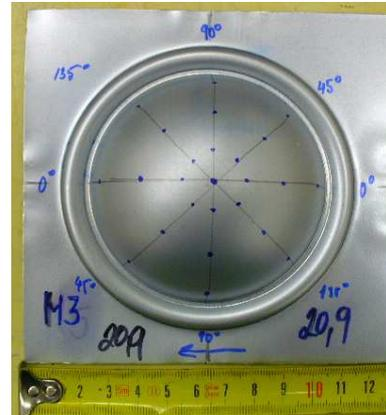
Fig. 2. Example tested specimens for HSLA H220PD steel sheet material (sample not burst)
