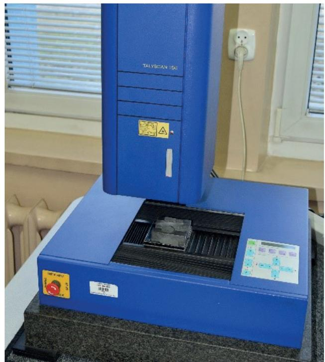
**Fig. 1.50.** TalyScan 150 dedicated to measurements of roughness
