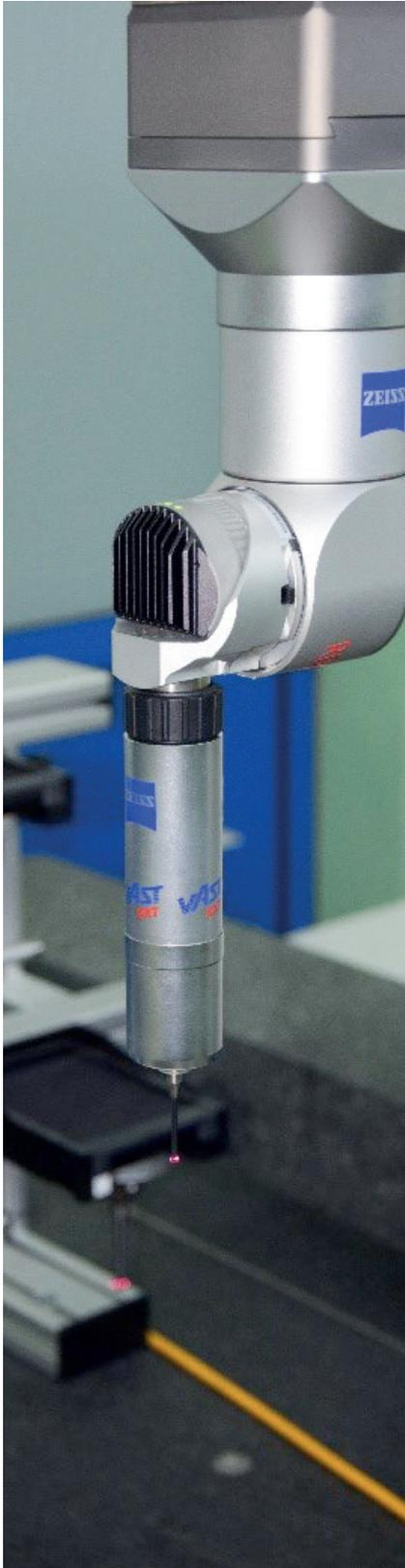
**Fig. 1.54.** VAST XXT contact measuring probe
