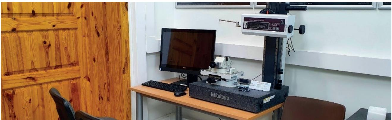
**Fig. I.40.** Test-stand for surface quality analysis at Kaunas University of Technology
