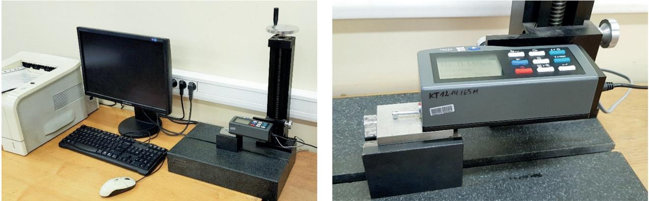
Fig. I.27. INNOVATEST Surface roughness tester TR-220
