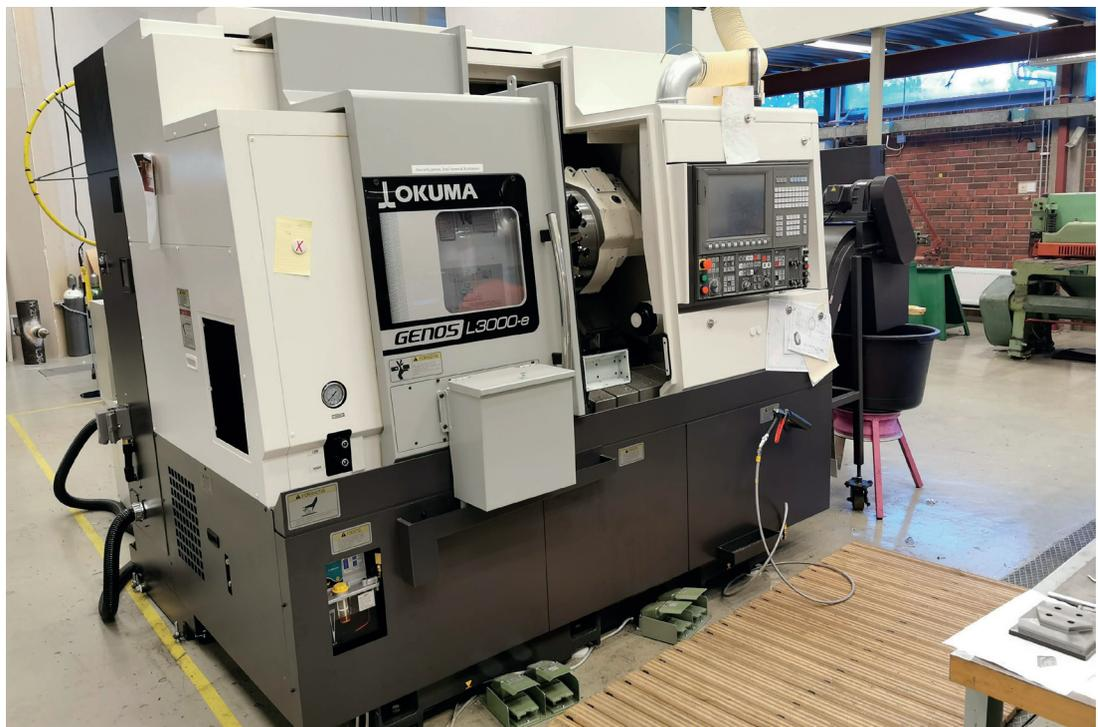
**Fig. I.60.** Okuma Genos L3000-e Horizontal Lathe
