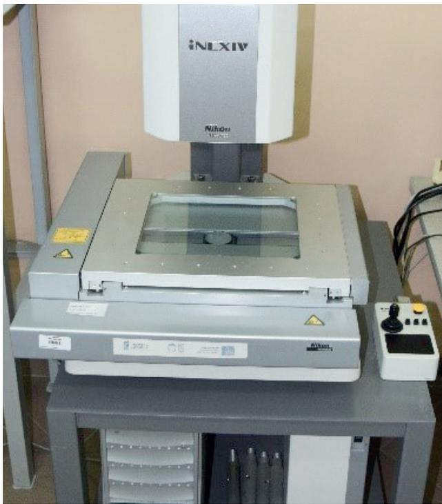
**Fig. I.44.** iNEXIV measuring system mainly dedicated to 2D non-contact measurements
