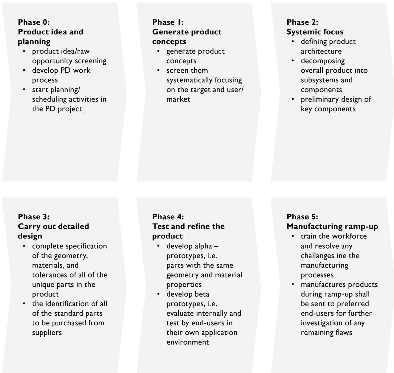
Fig. 2.2. Phases involved in product developing process
