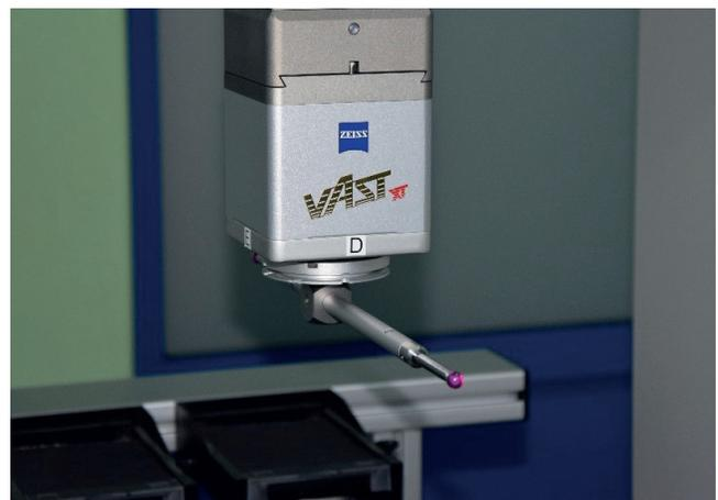
**Fig. I.53.** VAST XT contact measuring probe
