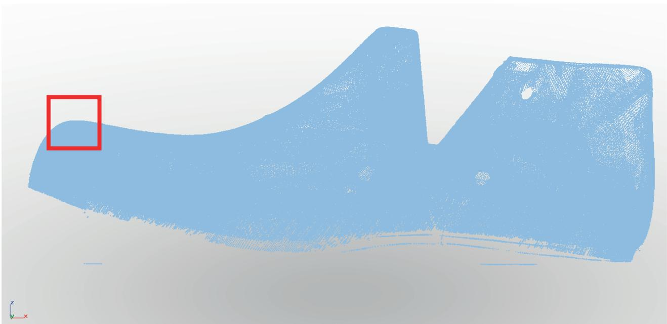
**Fig. I.9.** Point cloud representation of a physical object. Here there are close to 1 million points in the model
