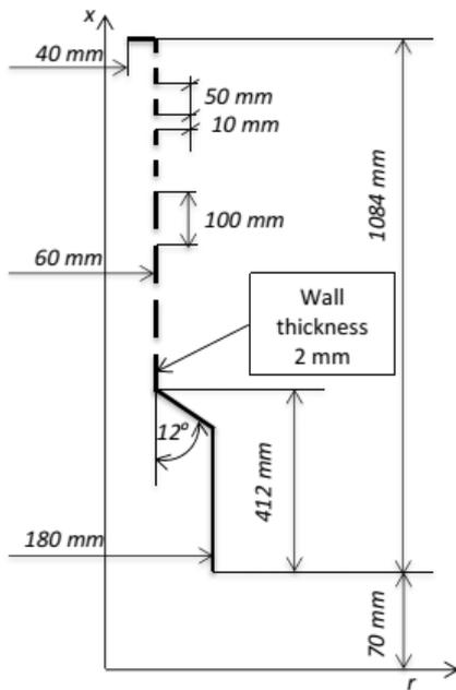
Figure 2. The stratification device geometry.
