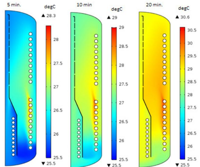
**Figure 5.** The temperature field in the tank after turn on the lower coil.
