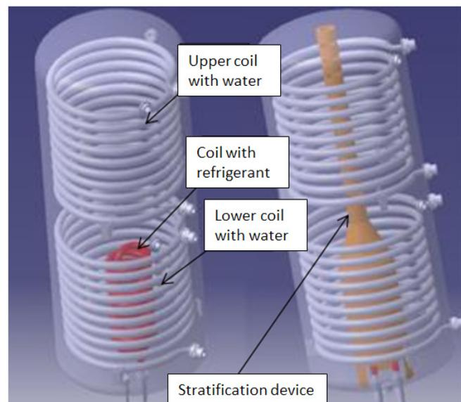
**Figure 1.** The geometry of the three-coil heat exchangers and the stratification device applied in the domestic hot water storage tank.
