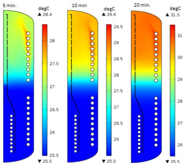
**Figure 6.** Temperature field in the tank during the operation of the upper coil
