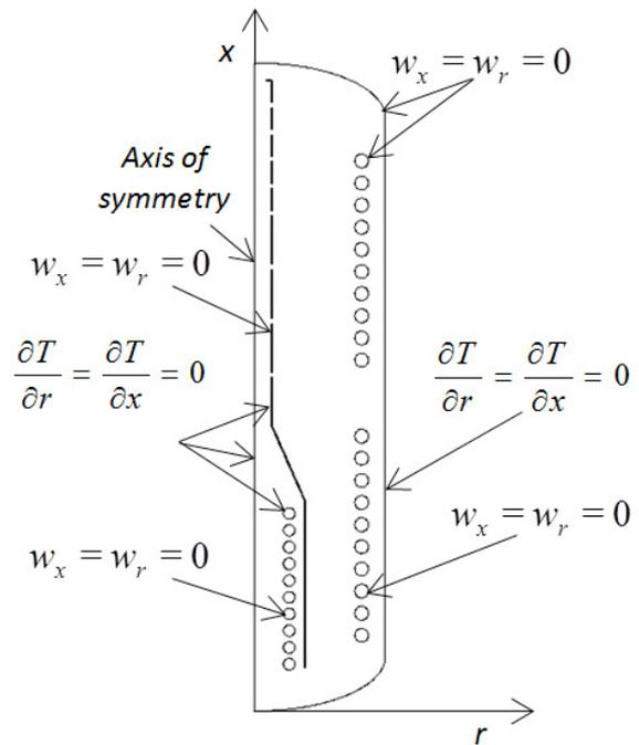
Figure 3. The 2D-dimensional computational domain for the storage tank with the boundary conditions specified on the wall of the tank, stratification device, coil with refrigerant, and the working coils with water.
