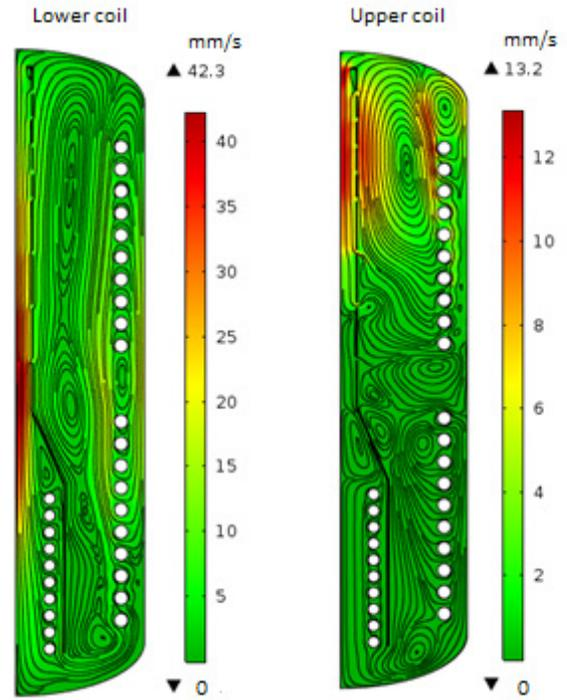
**Figure 4.** The 2D-dimensional velocity field and streamlines at 20 minutes after the turn on the coil.
