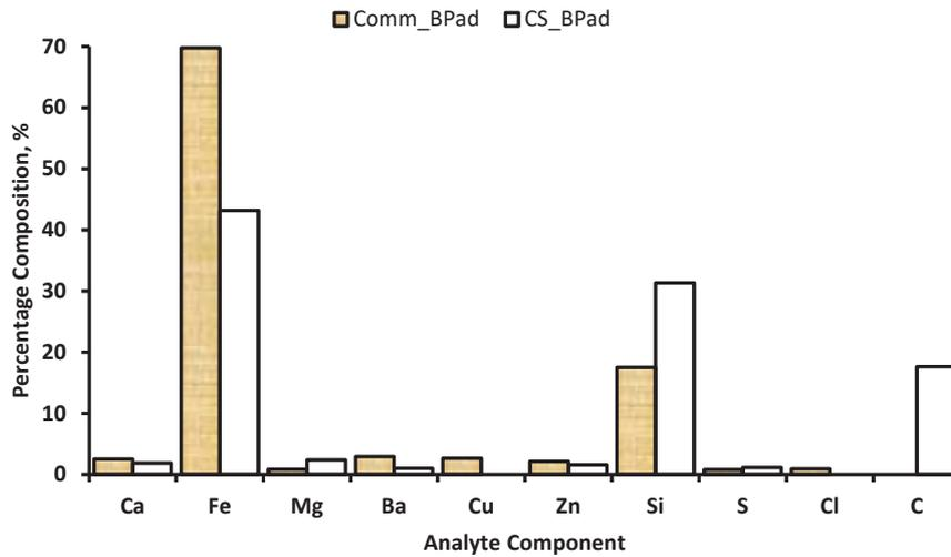
**Figure 9.** XRF analysis of control sample and CS-based samples with different grain size.
