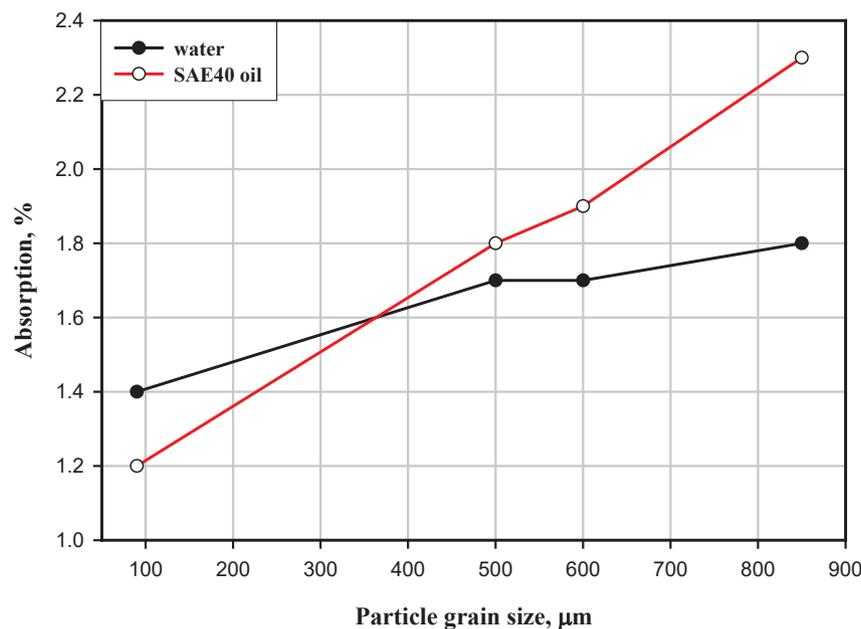
Figure 4. Water and oil absorption of CS-based brake pad samples with different grain sizes.
