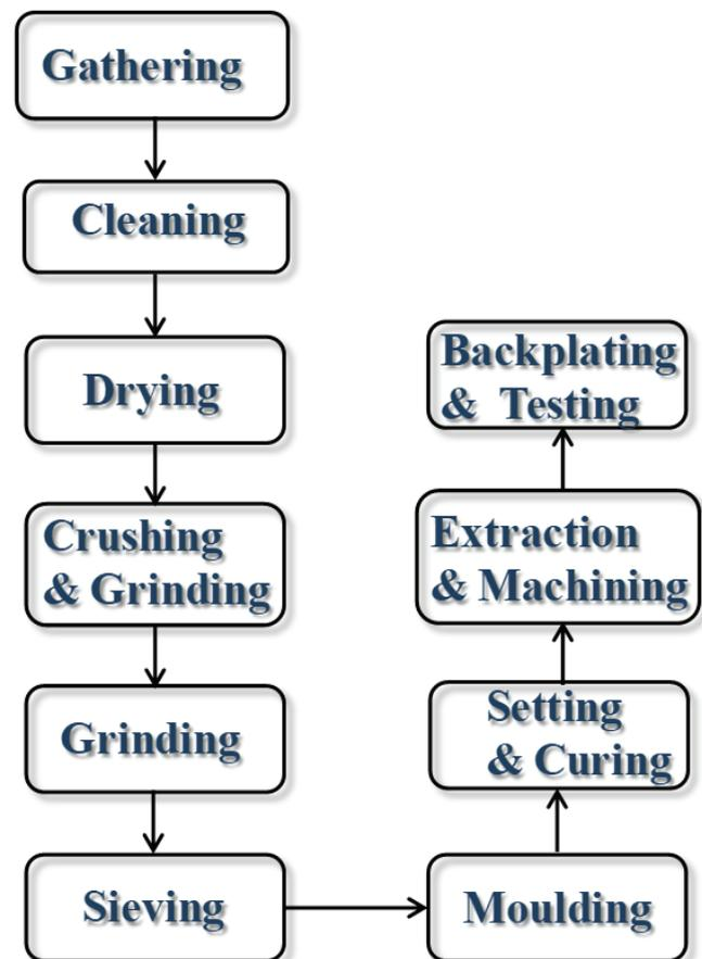
**Figure 2.** Procedure used to produce CS-based brake pad.
