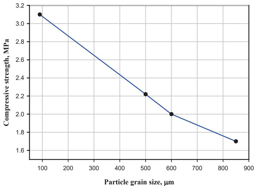
Figure 6. Compressive strength of CS-based brake pad samples with different grain sizes.
