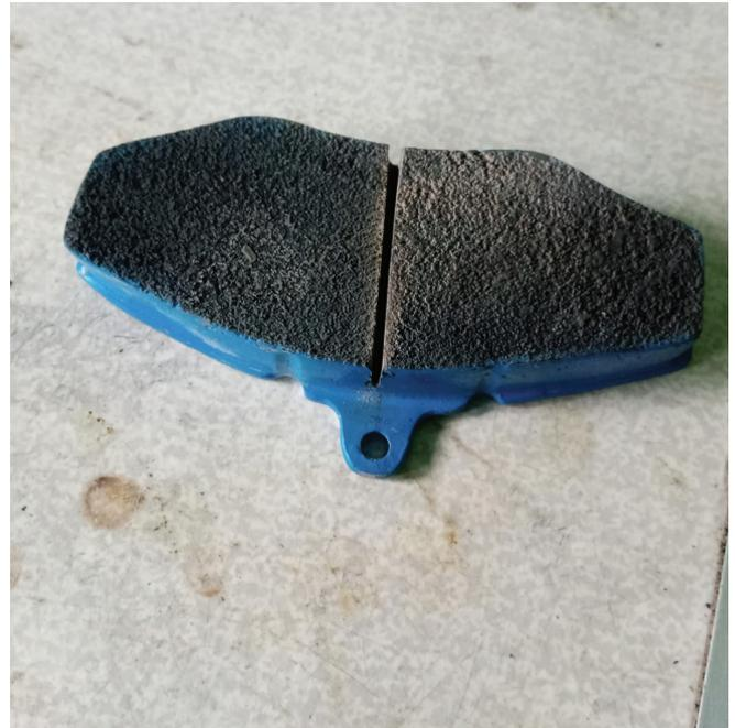
**Figure 10.** Finished CS-based brake pad sample.
