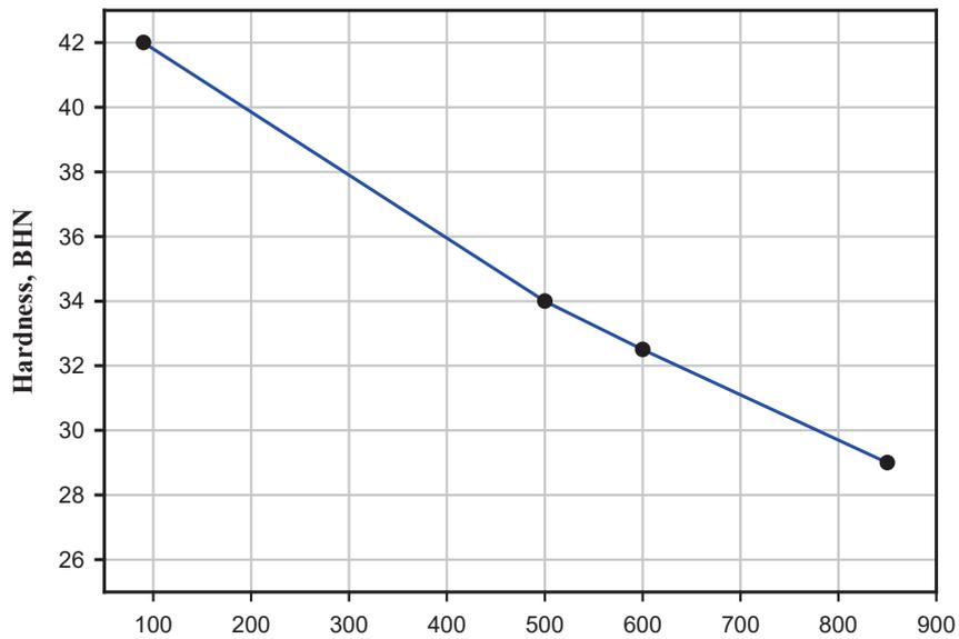
Figure 5. Brinell hardness (BHN) of CS-based brake pad samples with different grain sizes.
