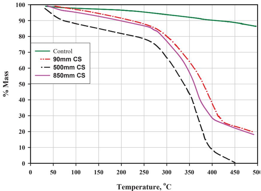
Figure 8. TGA results for the control and CS-brake pad samples of different grain sizes.
