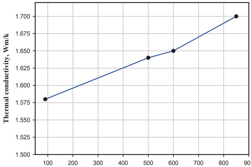
Figure 7. Thermal conductivity of CS-based brake pad samples with different grain sizes.
