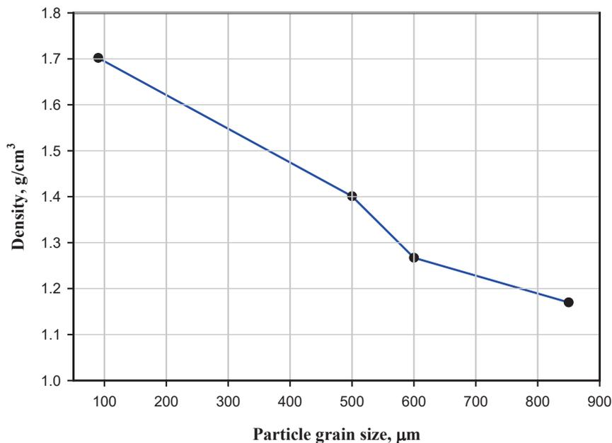
Figure 3. Density variation with particle grain sizes for CS-based brake pad samples.
