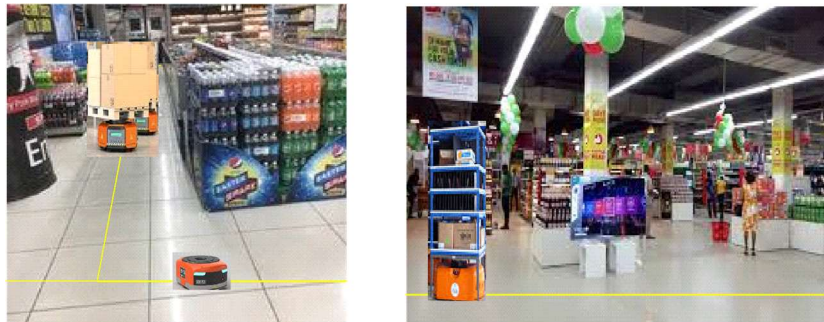
Figure 19. KIVA lifting shelves, racks, and crates on the run
