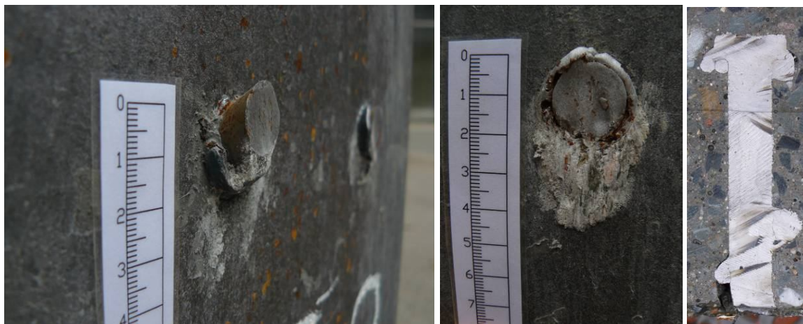
Fig. 11. Deformations base of shear connector in high-strength concrete
