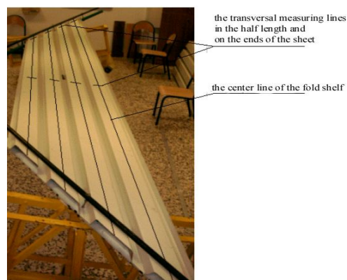
Fig. 11. An experimental free twisted trapezoidal sheet
