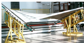
Fig. 1. Two free twisted sheets supported rectilinearly
