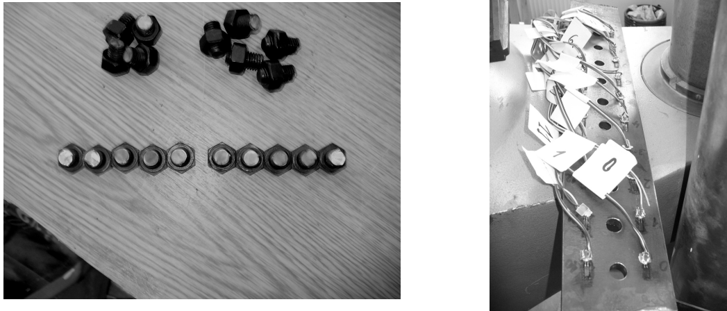
Fig. 5. Joint S960-02 after collapse
