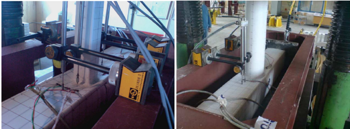
Figure. 1: Arrangement of the diagnostic apparatus on the specimens under observation
