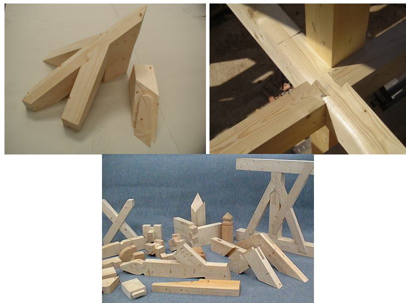
Fig.1. Various types of carpentry joints made by CNC wood-working machines – main advantage is an excellent accuracy of these connections
